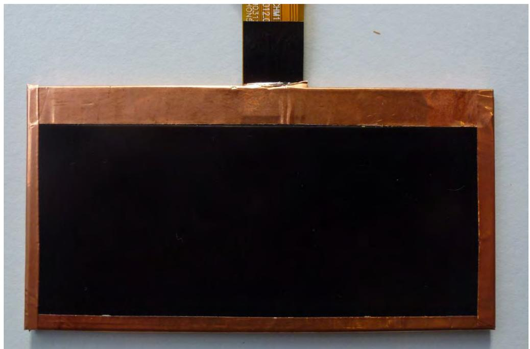
Fig 19. COG module with shielding around the module
