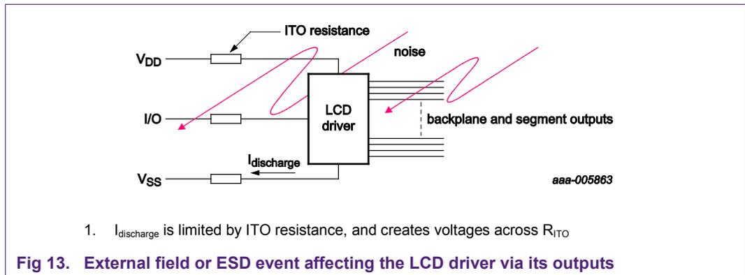
The discharge current will also flow via the V<sub>DD</sub> lines and I/O lines, but it is likely that most of the discharge current will flow via the V<sub>SS</sub> line. It is important to minimize the ITO track resistance, especially of the V<sub>SS</sub> line, in order to minimize the voltage step that results from these currents. These discharge currents will affect the supply voltage that the LCD driver sees, and the sudden change may affect the operation.
