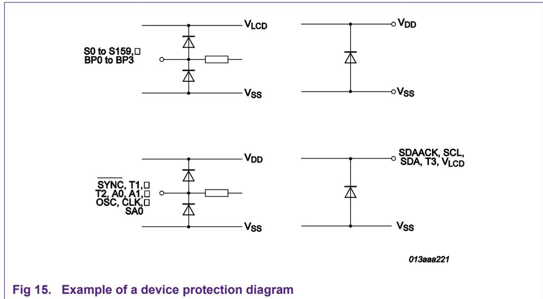
Fig 15. Example of a device protection diagram
