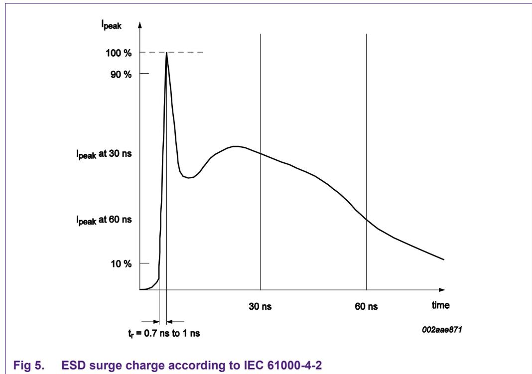
Fig 5. ESD surge charge according to IEC 61000-4-2
