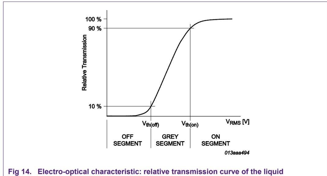
Fig 14. Electro-optical characteristic: relative transmission curve of the liquid
