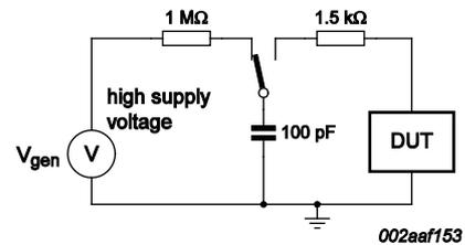
Fig 4. HBM test circuit (device level)
