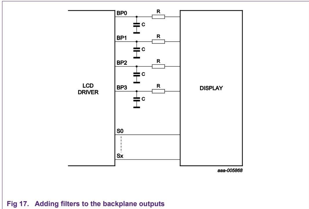
Fig 17. Adding filters to the backplane outputs
