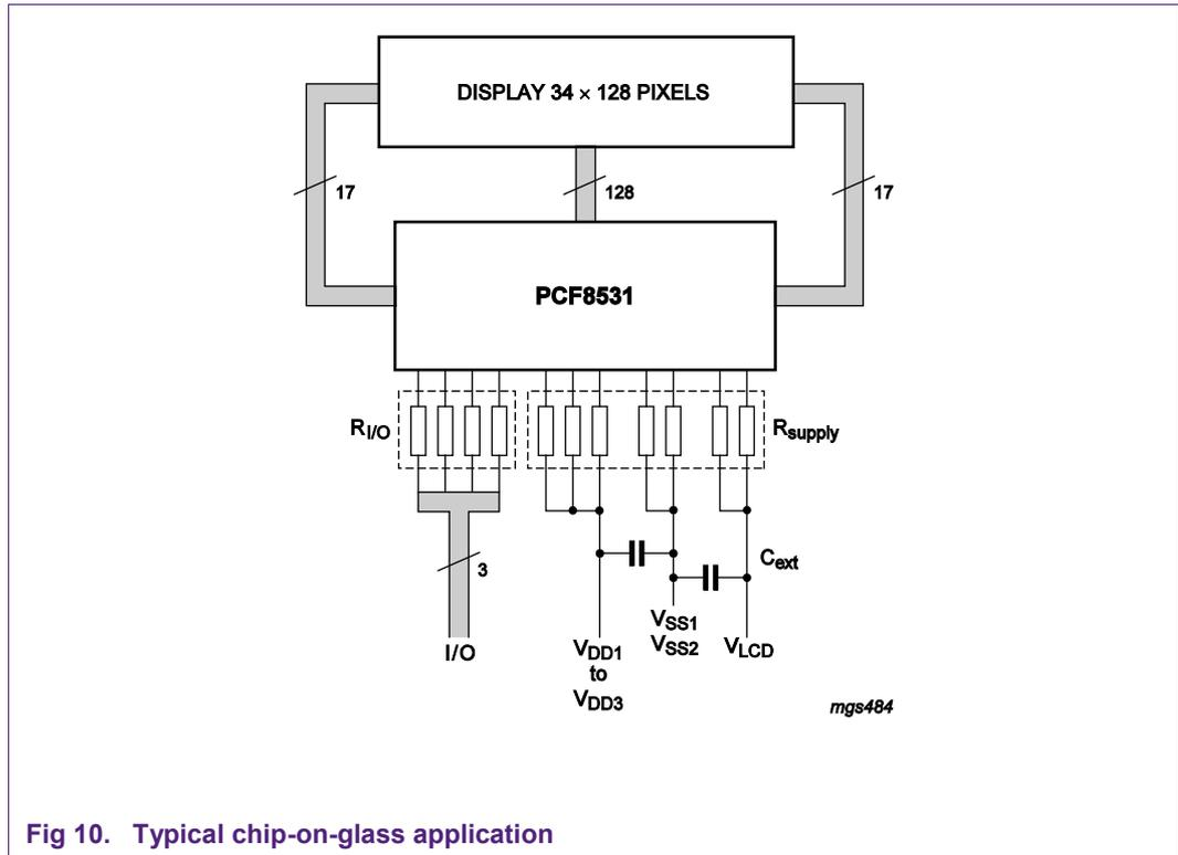
Fig 10. Typical chip-on-glass application
