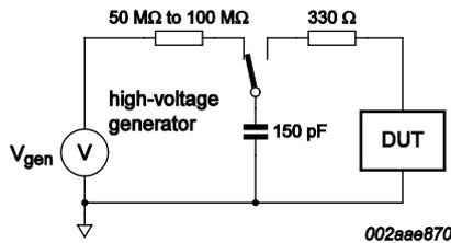
Fig 3. System level ESD testing according to IEC61000-4-2
