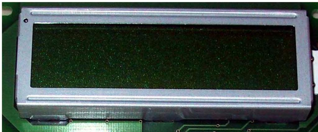
Fig 18. LCD with metal bezel
