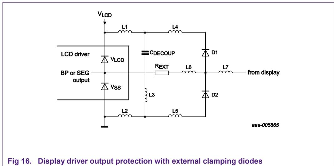
Fig 16. Display driver output protection with external clamping diodes
