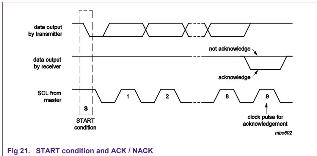
Fig 21. START condition and ACK / NACK
