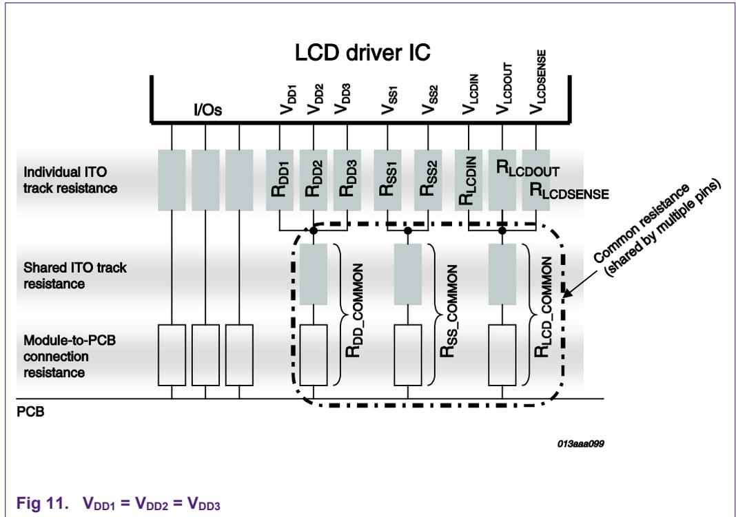
The  $V_{SS}$  line is most critical. Therefore the ITO track resistance has to be kept as low as possible.
