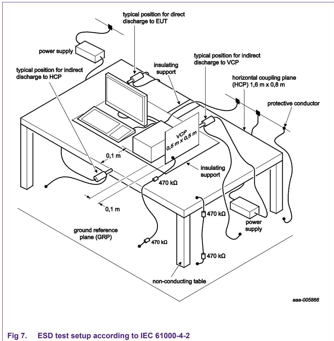
Fig 7. ESD test setup according to IEC 61000-4-2
