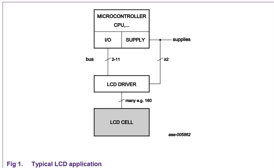
Fig 1. Typical LCD application
