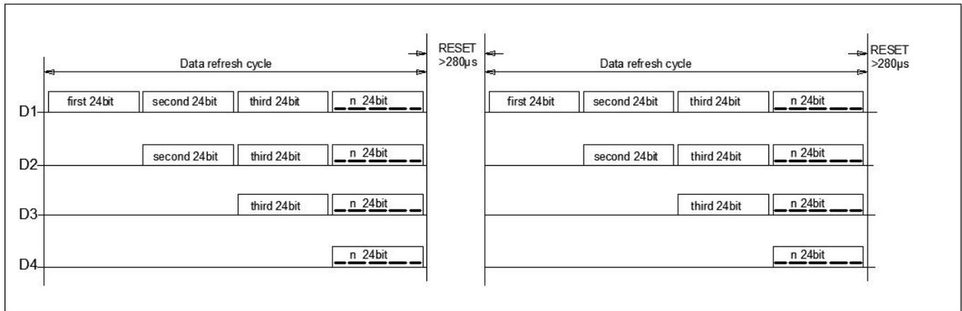
Note: The data of D1 is sent by MCU, and D2, D3, D4 through pixel internal reshaping amplification to transmit.
