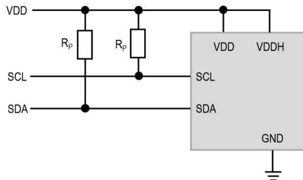
**Figure 1:** Typical application circuit (for better clarity in the image, the positioning of the pins does not reflect the positions on the real sensor). VDD and VDDH must be connected to each other close to the sensor on the customer PCB.
